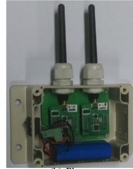
Fig. 3. Illustration of the multi-radio wireless communications module.
