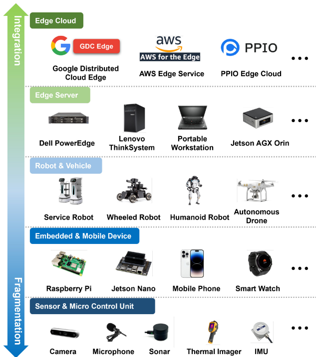
Fig. 5. The spectrum of edge networks can be classified into five categories: sensors and micro control units, embedded and mobile devices, robotics and Vehicles, edge servers, and edge cloud.
