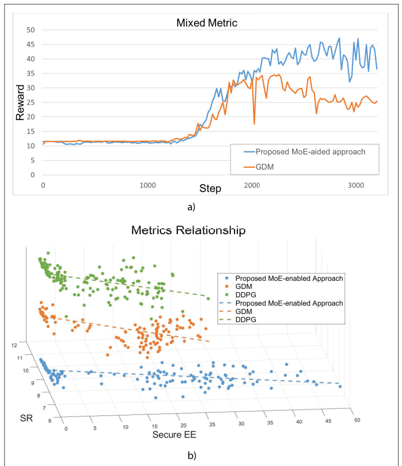
FIGURE 4. Performance comparison of three methods in the cooperative friendly jamming scenario: a) Comparisons of sum of Secrecy Rate and secure EE for three methods; b) Comparison of metrics relationship for three methods.
